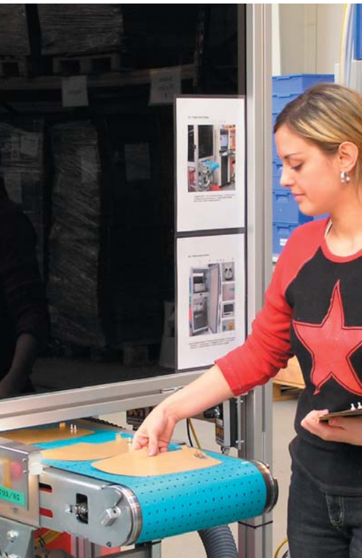
All foil elements are subjected to a pre-delivery optical inspection as performed here by Joanna Stanczewska (Backer OBR).
